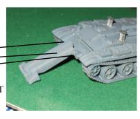
WITH THE HYDRAULIC RAM MOUNT LOOSE SO IT CAN PIVOT UP & DOWN
