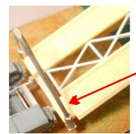
FIX THE 2 TIE BARS TO THE ENDS OF THE SBG SECTIONS. NORE 1 OF THEM HAS HOLES FOR THE 'A' FRAME
